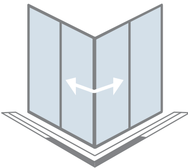
90° opening floating corner (sliding door leaves outermost)
